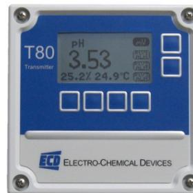
The Model T80 transmitter can be loop powered, 24 VDC powered or 100-240 VAC line powered. The standard configuration has a 4-20 mA output and a RS485 serial communication port with MODBUS® RTU output. A HART® communication version is also available. Alarm relays are optionally available on either line powered transmitter.
