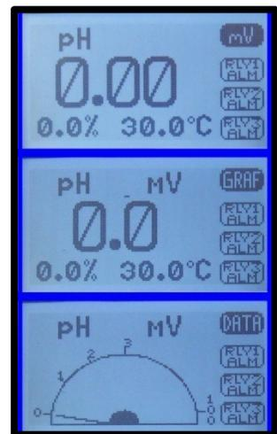
Each of the above screens also displays the condition of the optional Alarm Relays, black if energized and white if de-energized.
