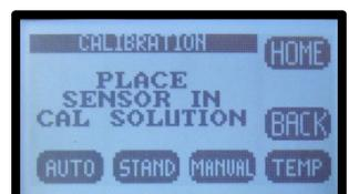
Any two solutions can be used for AUTO calibration however if solutions other than those listed above are used for calibration then the calibration values must be entered manually.
